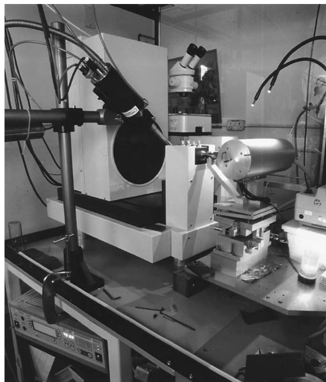
Figure 1 The MicroSource tube installed with a 30 cm MAR scanner.
